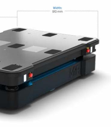
The MiR600 and MiR1350 are designed to comply with the highest available safety standards, making them superior to other AMRs. The two robots are the first IP52 rated AMRs in the market. This means that they have the ability to withstand dust particles and waterdrops and can be used in more challenging environments than other AMRs.
